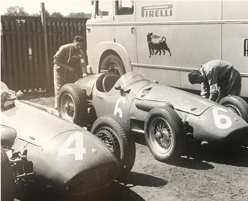
The line-up of cars with new louvreless bodywork. The car on the left is 2501, which first appeared in this form at the end of 1954; the other is 2515, one of the new cars for 1955. ( Ferret Fotografics )
